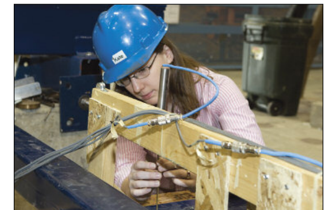
UMaine graduate student Kate Beaumont adjusting LVDT to measure sample displacement during a boat hull structural test.
