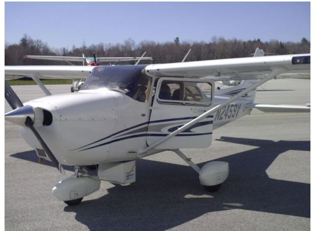
University of Maine graduate student Dave Sandilands flew this Cessna 172 over the Orland transfer station site to take pictures for an aerial survey. The camera is mounted in a box on the plane’s belly.
